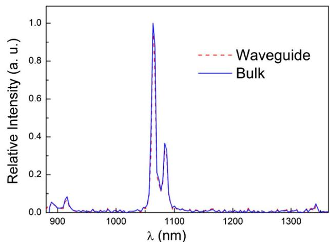
Fig. 3. Room-temperature luminescence spectra obtained from the waveguide (red-dashed line) and bulk (blue solid line) at the room temperature pumped by the laser at the wavelength of 808 nm.
