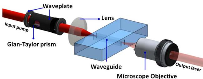
Fig. 1. Experiment setup for the self-Q-switched waveguide laser generation.
