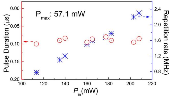
Fig. 6. Variation of the pulse duration and the repetition rate of the self- $Q$ -switched pulse waveguide laser as a function of the input pumping power.
