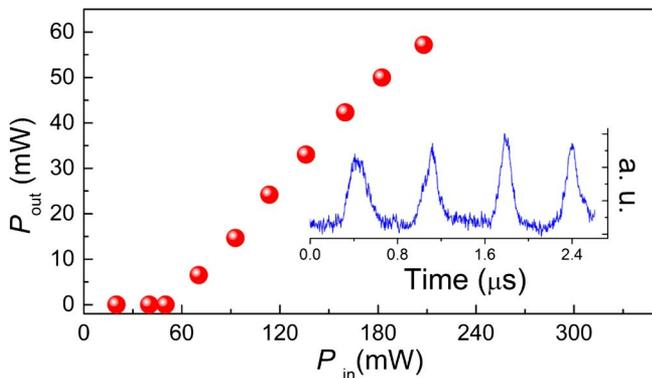
Fig. 5. Output power of 1064 nm laser as a function of the absorbed pumping power at 808 nm. The pulse train of pulsed laser is shown in the inset with the pumping power of 160 mW.
