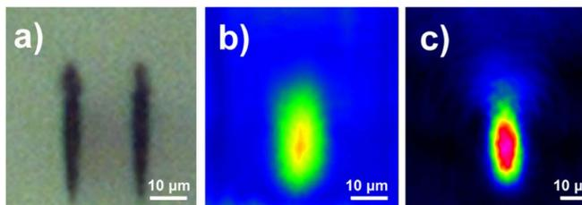
Fig. 2. (a) Cross sectional microscope image of the inscribed Type II waveguide in the Nd:Cr:YVO<sub>4</sub> crystal; the measured modal profile of (b) the pumping laser at 808 nm and (c) the output laser at  $\sim$ 1064 nm.
