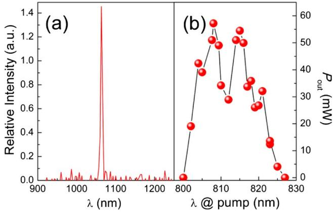
Fig. 4. (a) Laser oscillation spectra of the self- $Q$ -switched waveguide laser. (b) Maximum power of the output laser as a function of the wavelength of the pumping laser with  $\pi$  polarization.
