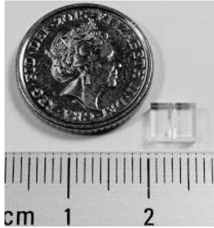
Figure 4.11 Optofluidic device in fused silica: Dimension 6 \times 4.8 \times 2 mm. The chip dimension compared with 5 pence coin.
